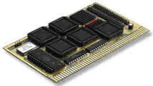
With the FastATA 4000 MK-V controller you can take advantage of the latest low-cost, high-capacity ATA/EIDE devices like hard drives, CD-ROM drives, CD-RW drives, ZIP drives, LS-120 drives, etc. The minimum hardware configuration is: Amiga 3000 or Amiga 4000. The recommended configuration is: Amiga 3/4000 with 68060 (or PPC with 68060) processor card with 64MB RAM.
